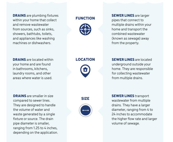
Drains are smaller pipes within your home that collect wastewater. Sewer lines are larger pipes that connect multiple drains and transport the combined wastewater away from the property.
